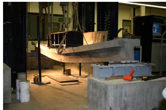
Figure 3: Testing the Control T Specimen
