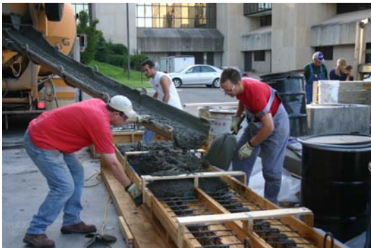
Figure 2: Casting of the T Specimens
