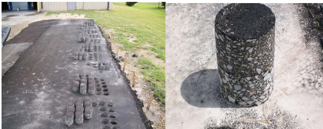
Figure 2: The core samples after being removed from the pavement
